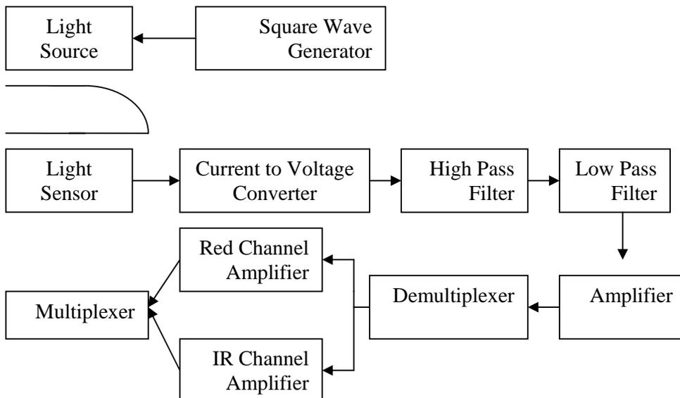
1. The finger is inserted between LED's on one side and the photo-diode sensor on the other side. External light interference is minimized by covering the assembly by black material.
