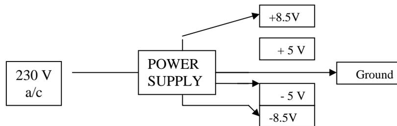
1. It is designed to supply regulated  $\pm 8.5V$  for the analog IC's and  $\pm 5V$  for the digital circuitry.
