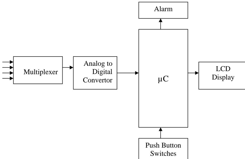
1. Atmel 89C52 Microcontroller with 8kb internal memory and  $16 \times 2$  LCD display is used.
