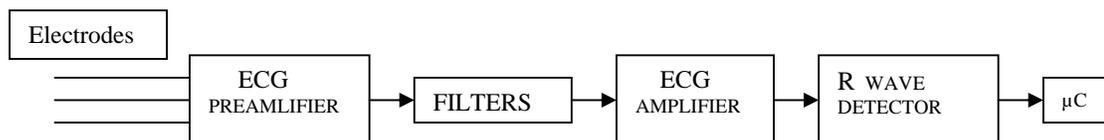
1. The ECG signal is obtained from chest electrodes using 3-lead system.
